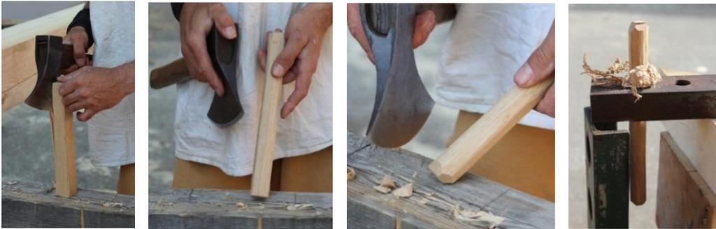
Fig. 15 Process of dowel manufacture
