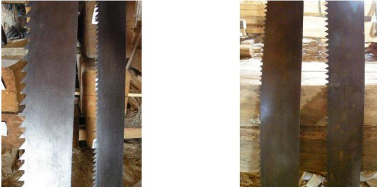
*Fig. 39 Saw band for longitudinal cutting (left), saws band for cross cutting (right)*
