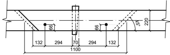
2.2.2.4 Two-key joint with oblique undercut faces secured with one dowel
