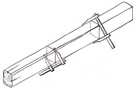
Fig. 11 Measuring the minimum diameter of the log at waness
