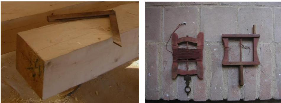
*Fig. 40 Bevel gauge (left), chalk line with clay (right)*
