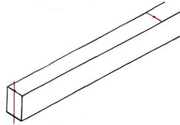
Fig. 19 Plotting the rough length of the scarf joint and marking the end point of the top surface
