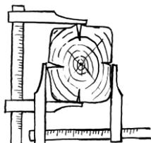
*Fig. 13 Taking into account deformation when measuring the section*
