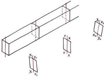
Fig. 18 Dividing the beam section into two equal halves taking into account possible twisting
