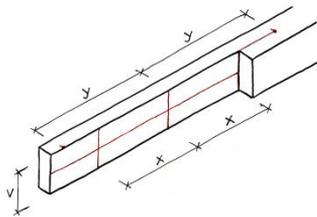
Fig. 24 Measuring the scarf joint length
