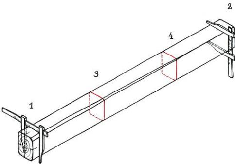
Fig. 10 Measuring the original beam section at four places
