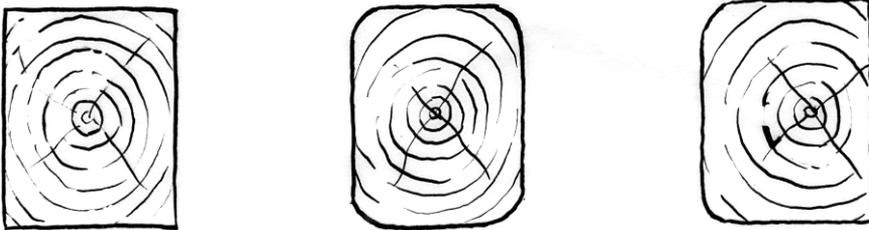
Fig. 12 a) Centric sharp-squared section, b) centric section with waness, c) eccentric section with waness on one side of the member
