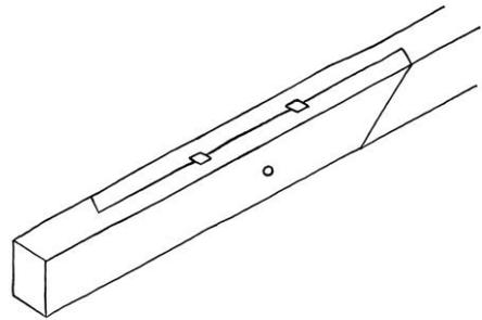
*Fig. 36 Scarf joint after assembly and finishing*
