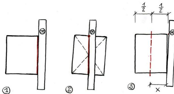
Fig. 17 Exact method of beam section measurement; 1 - determining the inclination in the middle of beam, 2 - plotting the axis of the cut on the cut off face, 3 - location of the point of the second division point at the end of the scarf joint
