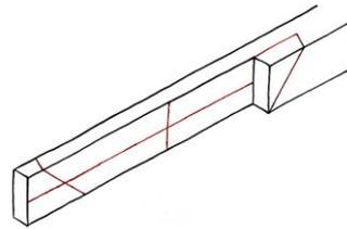
Fig. 26 Plotting the lines of the oblique undercut face
