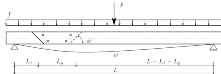
Fig. 9 Dimensions of structure and beam deflection (above), dependence of beam stiffness with a joint shifting along the beam centreline (bottom)
