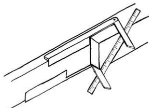
Fig. 25 Plotting the lines of the cross cut of the joint faces
