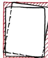
*Fig. 14 Taking into account twisting when measuring the section*
