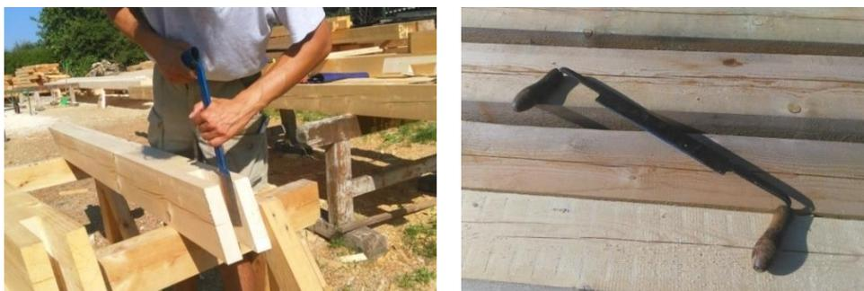
*Fig. 38 Chisel axe (left), drawknife (right)*
