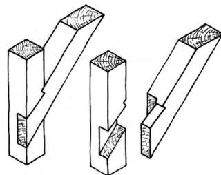
Fig. 5 Dovetail lap joint [2], [50]
